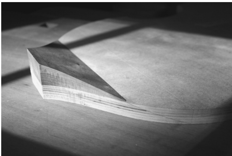
Figure 9. The shoulder portion of a viol form built according to the interpretation of Diderot's false table presented in this paper. The pencil line shows how the angle of the fold begins at the bottom of the form and extends to the surface of the wedge. The sides below the pencil line will later be cut away to create the angle of the fold.
